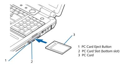
Figure 4-8. Installing/Removing PC Cards
